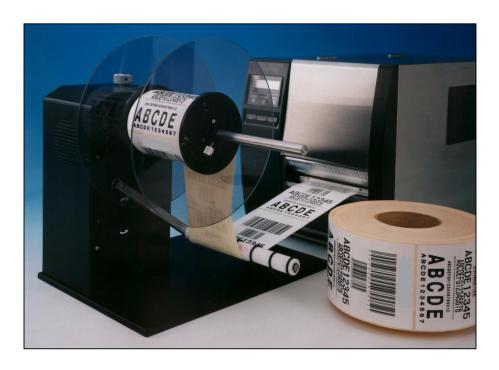
For high volume rewinding, the UR100 Universal Rewind Unit is suitable for most makes of thermal printer. Its dancing arm and reversible motor enable the UR100 to rewind labels inside or outside wound onto various core sizes.
